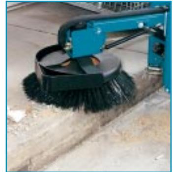
While the main brush sweeps debris on street level, the SB2 cleans up on the curb.
