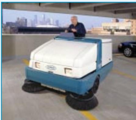
Optional dual side brushes allow the 6650XP to clean both sides of parking ramp entrances and exits—with the flow of traffic.
