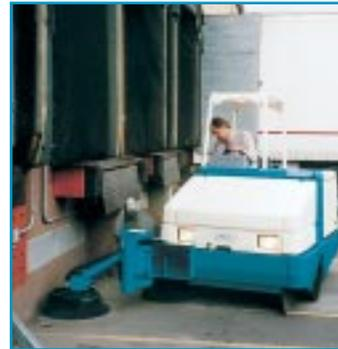
The Model 6650's optional SB2 auxiliary sidebrush cleans areas not accessible to regular sweepers.
